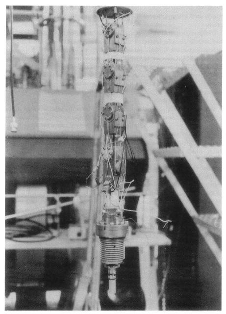
Figure 2: Photograph of the lower portion of the dilution refrigerator used in the discovery, showing the heat exchange column and, at the bottom, the mixing chamber with the <sup>4</sup>He bellows chamber and piston for the Pomeranchuk cell attached.
