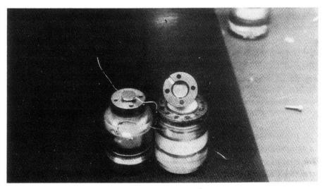
Figure 3: Photograph of the capacitive pressure transducer for the <sup>3</sup>He cell during assembly. The moving capacitor plate attached to the metal diaphragm is seen at the left, while the stationary plate is on the right.
