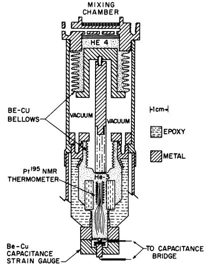
Figure 1: Schematic diagram of the Pomeranchuk cell used in the discovery of superfluidity in <sup>3</sup>He. Superfluid <sup>4</sup>He is added to the upper bellows assembly under pressure, forcing the lower bellows into the <sup>3</sup>He-filled region. The capacitive pressure transducer is at the bottom. (Reproduced with permission from reference 11).
