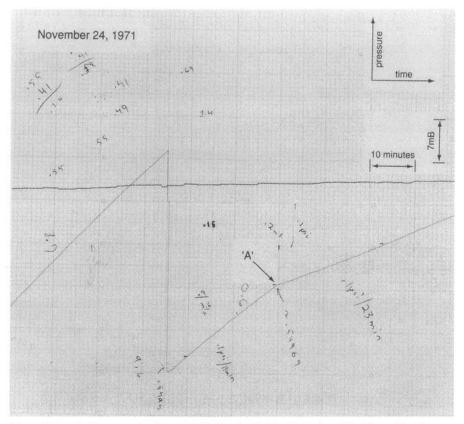
Figure 4: Pressurization curve taken Nov. 24, 1971, showing the first observation of the 'A' transition. Pressure increases vertically while time increases to the right. The abrupt jumps in the pressurization curve occurred when the capacitance bridge was re-balanced. The ragged line is the temperature of the dilution refrigerator.
